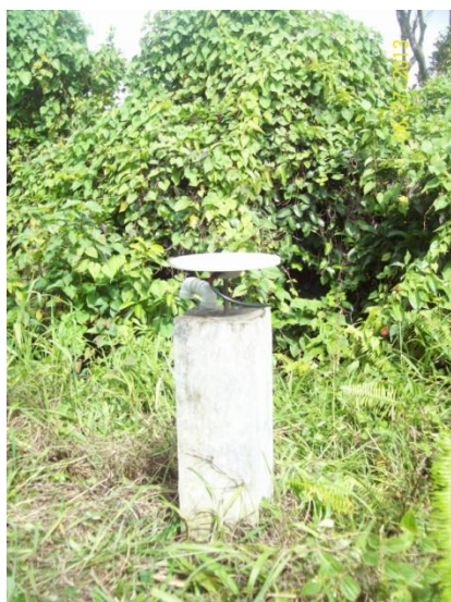
Figure 31 This is a permanent GPS station maintained by the University of the West Indies. We visited this site to address data transmission issues likely due to vegetation overgrowth.
